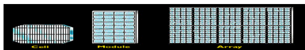
Fig.3.6 Cells are assembled into modules, which are further assembled into arrays. (U.S. Department of Energy Photovoltaic's Program)
